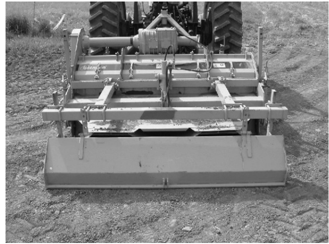
Fig. 2. Power hiller set to form a 1.8 m wide bed.
