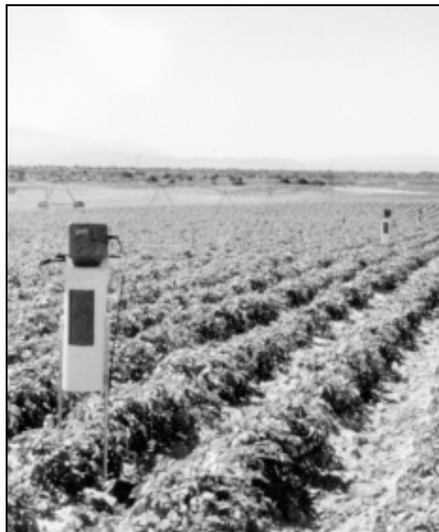
Soil moisture sensors in an eastern Idaho potato field.
